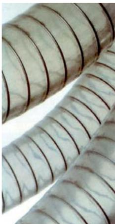
Transparent flexible PVC hose reinforced with steel spiral embedded in the wall, for the suction and discharge of fluids containing material.
